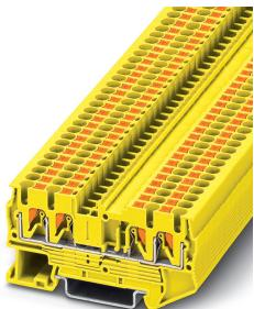
Feed-through terminal block, nom. voltage: 800 V, nominal current: 24 A, connection method: Push-in connection, 1 level, Rated cross section: 2.5 mm<sup>2</sup>, cross section: 0.14 mm<sup>2</sup> - 4 mm<sup>2</sup>, mounting type: NS 35/7,5, NS 35/15, color: yellow
